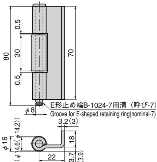
参考取付け例 Example of installation (Reference)
